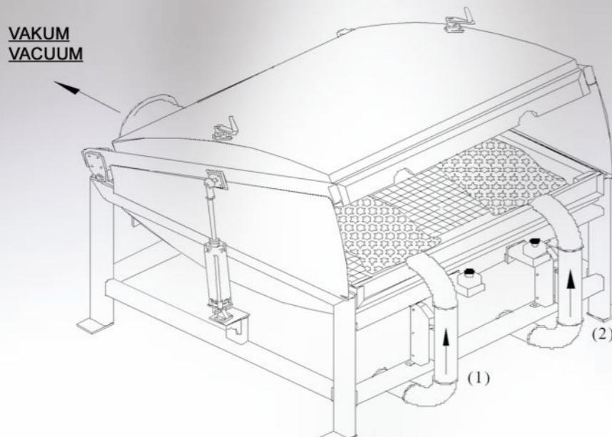
From C40 weighing machine weighed fiber transferred by vacuum suction through the fabric cover. With C45 Pillow Filling machine can fill the fibers to the pillow cases, cushions or furniture covers automatically with uniform distribution of fibers including in the corners.
